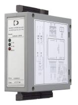
The SAB-S-MODBUS is a two-channel module that measures single or multiple magnet transducer position and returns this information to a host computer via a serial interface using the Modbus ASCII or RTU protocol over a RS232 or RS485 port. Communication setup is controlled via dip-switch settings and sensor interface configuration is controlled via Modbus registers.
